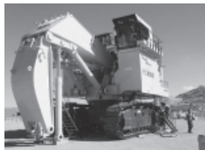
One of two 23 cubic meter hydraulic shovels.
